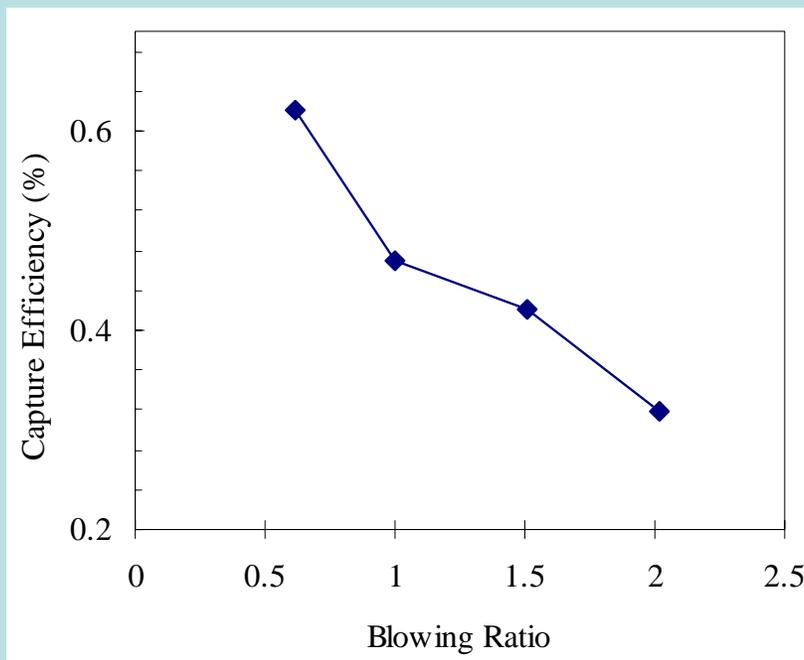
**Testing Conditions:** Inconel alloy, 3-cylindrical holes,  $d=1.5$  mm,  $3d$  spacing,  $M=0.6, 1.0, 1.5, 2.0$ ; 4 hr tests, Density ratio=1.8-2.3
