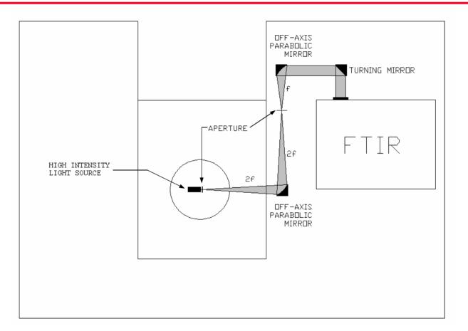
A high intensity fiber optics light is directed through an aperture positioned in the location of the probe. The result is a point source of visible light that follows optical path.
