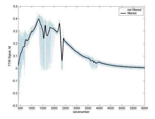
The emission signal measured by the FTIR from a layer of deposited ash on the probe.
