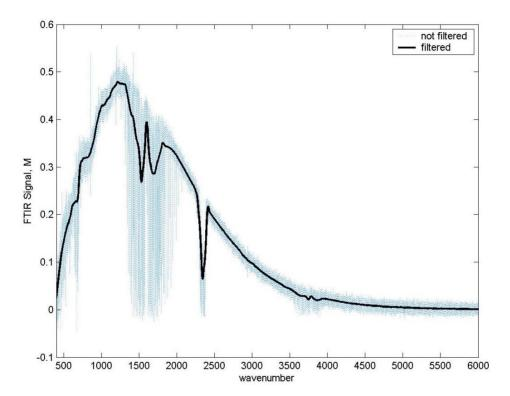
Filtered emission signal from black body radiator at 465° C. The filtering scheme fits quadratic curves over a large number of small intervals.
