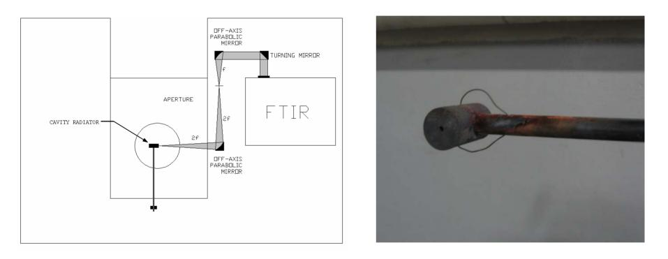
The effective emittance of a cavity radiator will be calculated and compared to the measured emittance.
