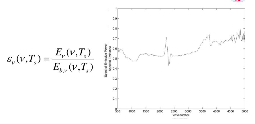
The spectral emittance of the ash deposit is the ratio of the spectral emissive power of the ash deposit to the black body emissive power at the same temperature.
