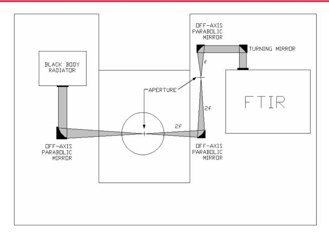
The radiative energy of a black body radiator is focused to the probe location, resulting in a point source of black body radiation that follows the optical path.
