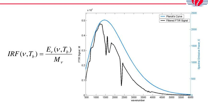
The instrument response function (IRF) provides a relationship between the signal measured by the FTIR and the emissive power of the source.
