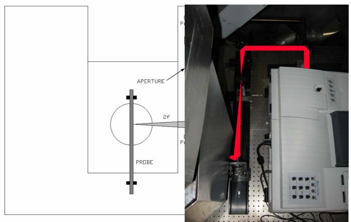
Optical path used to collimate the radiative energy from the deposited ash on the probe and direct it into the Fourier Transform Infrared Spectrometer (FTIR Spectrometer).
