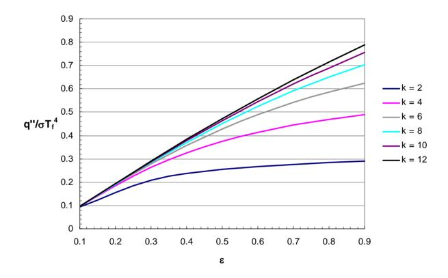
Effect of emittance and thermal conductivity of ash layer on heat flux.
