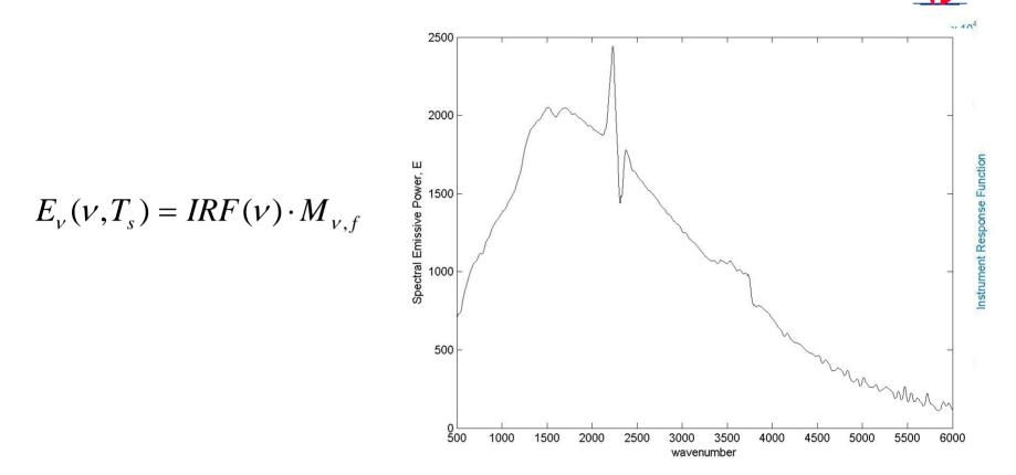
The spectral emissive power of the ash deposit can be found by multiplying the FTIR signal by the IRF found during the calibration process.
