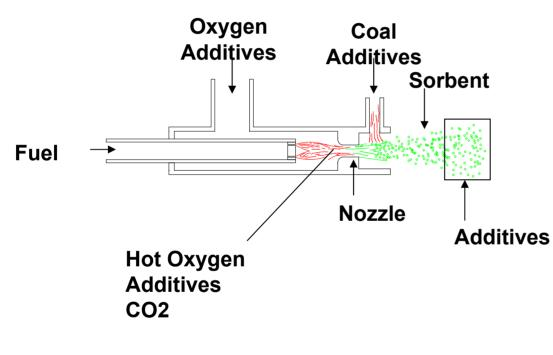
Patented burner is the basis of the PAC production process
