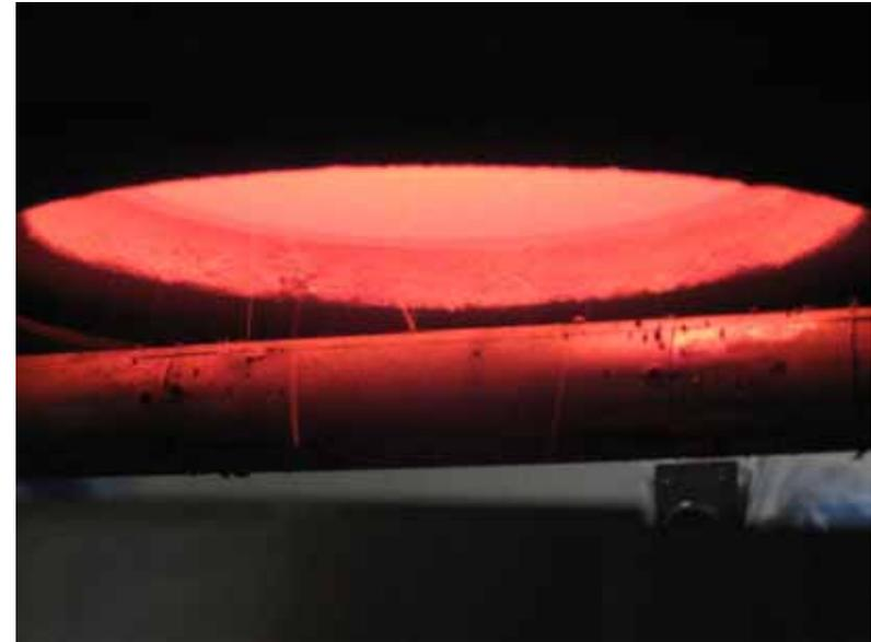
Deposition tube collecting deposit at reactor outlet
