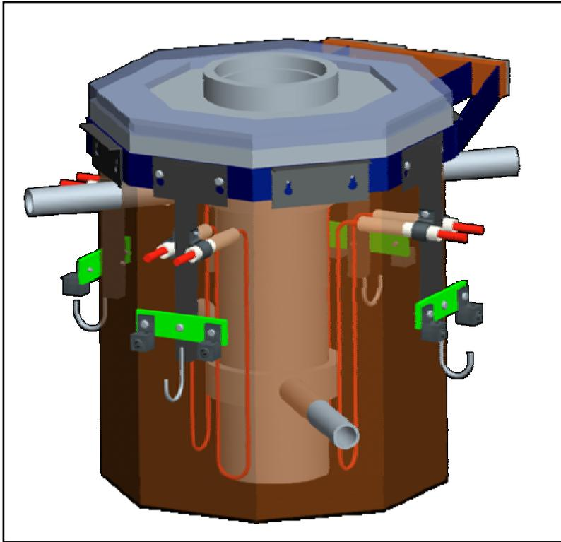
One of Seven Sections in the Heated Multi-fuel Reactor
