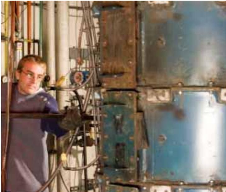
Burner Flow Reactor – Realistic burner fluid flow, 25 kg/hr coal
