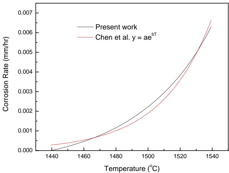
Comparison of corrosion rate calculated using the present model and the Chen et al. equation
