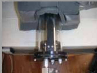
FTIR gas cell chamber. Path length of 10 m
