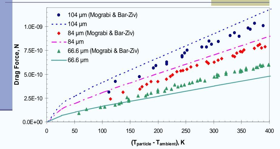
Comparison of Fluent<sup>™</sup> predictions with experimental results of the free-convective drag force (Mograbi & Bar-Ziv, 2005)
