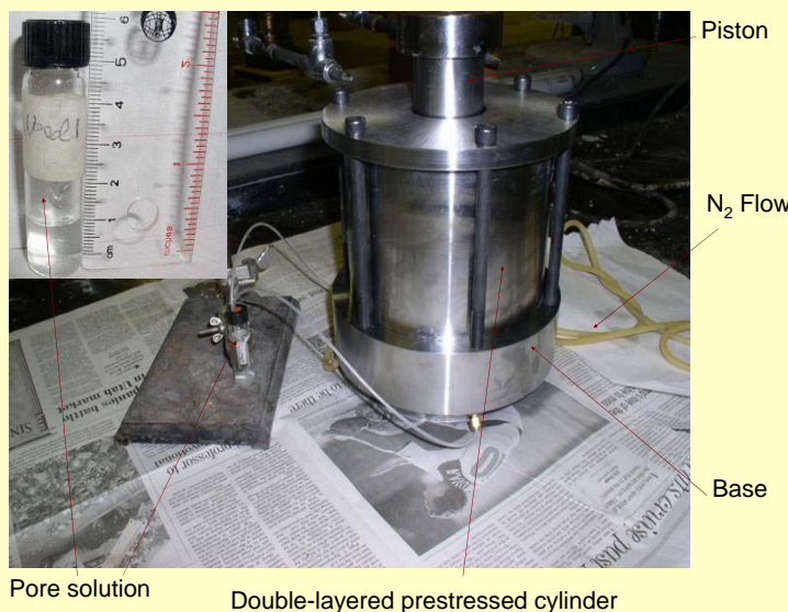
Expansion Measurement ( \pm 0.0001\text{in} )
