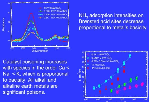
Catalyst poisoning increases with species in the order  $\text{Ca} < \text{Na} < \text{K}$ , which is proportional to basicity. All alkali and alkaline earth metals are significant poisons.
