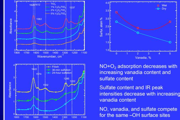
$\text{NO} + \text{O}_2$  adsorption decreases with increasing vanadia content and sulfate content
