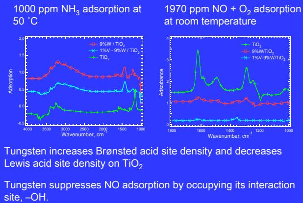
Tungsten increases Brønsted acid site density and decreases Lewis acid site density on  $\text{TiO}_2$
