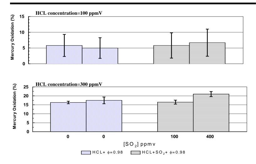
SO<sub>2</sub> has little effect on oxidation by HCl
