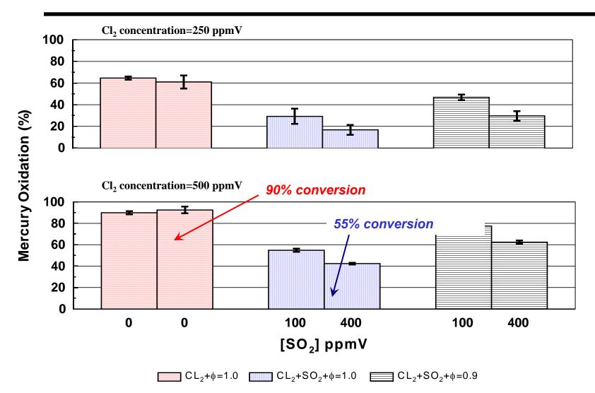
SO<sub>2</sub> suppresses oxidation by Cl<sub>2</sub> under all conditions
