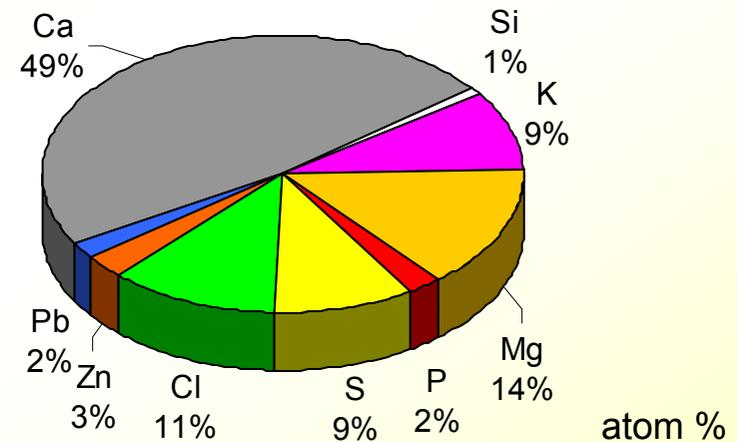
Coarse fly ash particle from the combustion of bark
