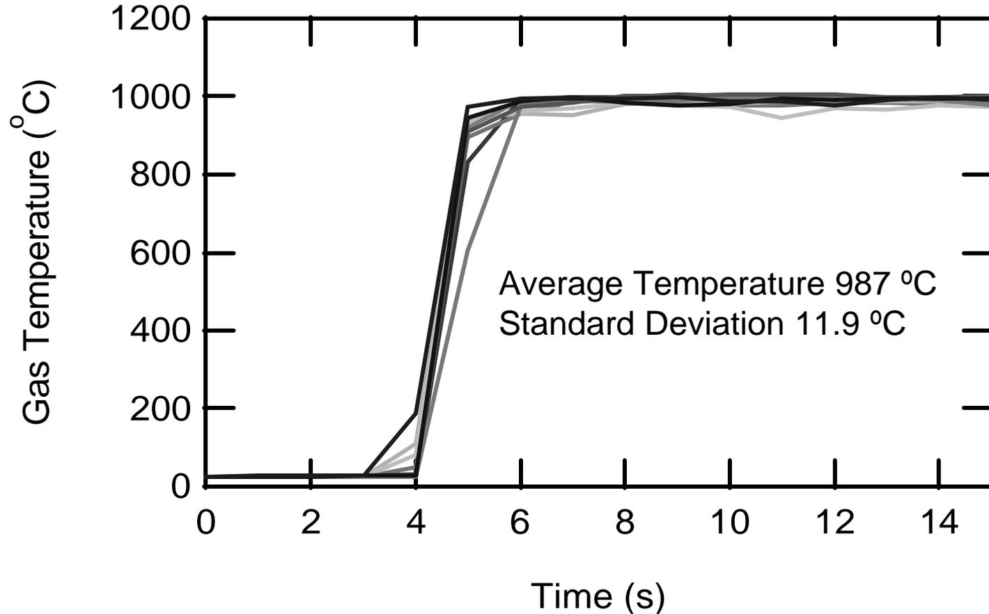
\*127  $\mu\text{m}$  diameter type K thermocouple 2" above the FFB
